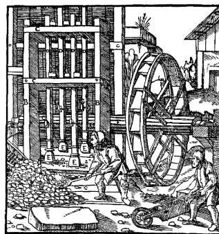
A—MORTAR. B—STRAIGHT POST. C—CROSS-BEAM. D—CRANK. E—TRUCK HEAD. F—AXLE (CAM-SHAFT). G—TOOTH OF THE STAMP (TAPPET). H—TEETH OF AXLE (CAM).
